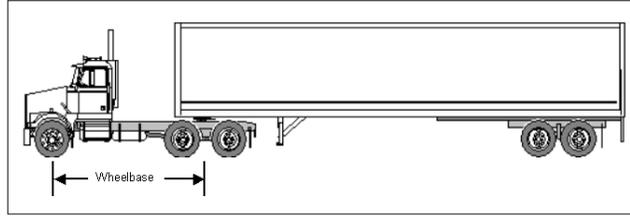
**Figure 7: Tractor Wheelbase**
