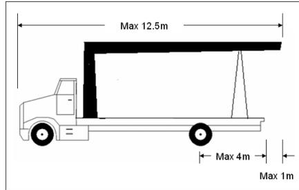
**Figure 6: Overhanging Boom of a Rear-Facing Crane**
