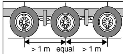
The allowable weight is determined from Table 2 based on the spacing between the first and last axle.
