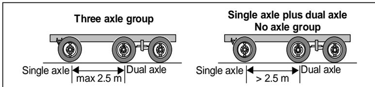
The allowable weight is determined from Table 4 based on the spacing between the first and last axles.
