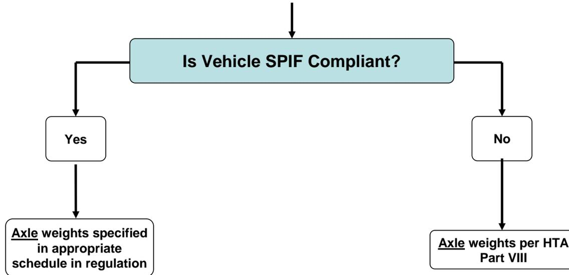
FLOWCHART TO DETERMINE APPROPRIATE WORKSHEET FOR ALLOWABLE GROSS WEIGHT
