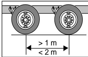
The allowable weight is determined from Table 3 based on the spacing between the two axles.
