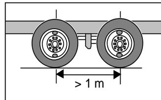
The allowable weight is determined from Table 1 based on the spacing between the two axles.
