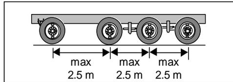
The allowable weight is determined from Table 5 based on the spacing between the first and last axle of the group.
