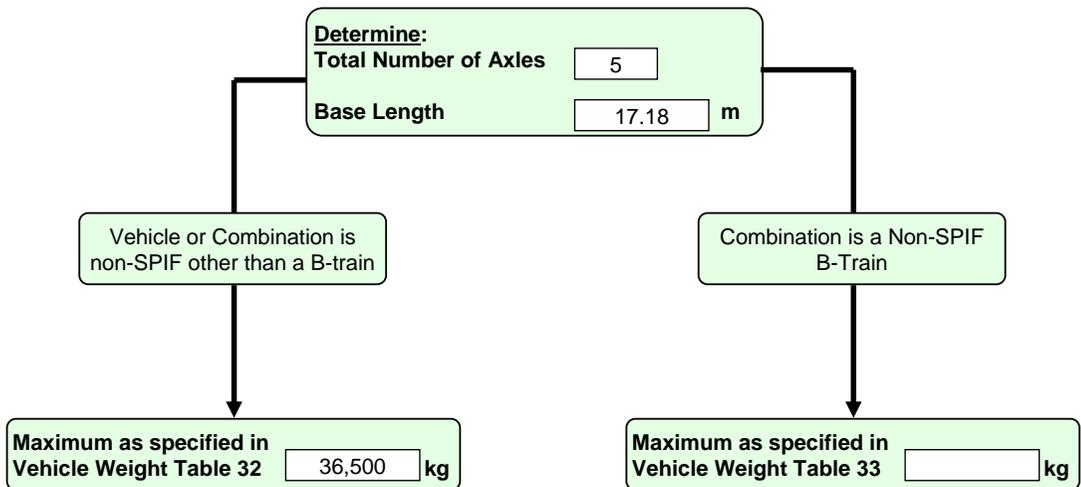
The non-dump semi-trailer in this example is equipped with a rigid air-lift axle which disqualifies the combination from being SPIF. Other than dumps or tankers, all grandfathering protection for non-SPIF semi-trailers with 3 or less axles has expired.
