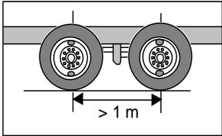
The allowable tandem drive axle weight for a 3-axle tractor is determined from the table based on the spacing between the two axles.
