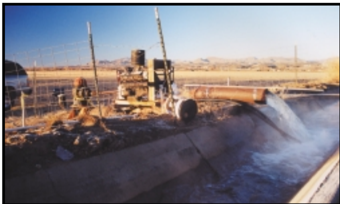
Running of a 24-hour pump test at a local farmer's irrigation well near San Antonio, New Mexico. Photo by Laura Wilcox, February 2002.
