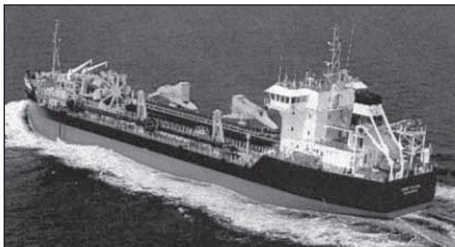
Figure 7. Modern dredger with bucket wheel discharge facilities (Courtesy RMC Group).
