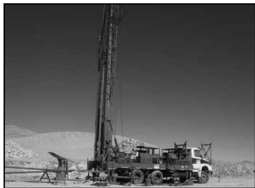
Figure 8. Direct rotary drill rig for mud-rotary drilling, western Salta Province, Argentina.
