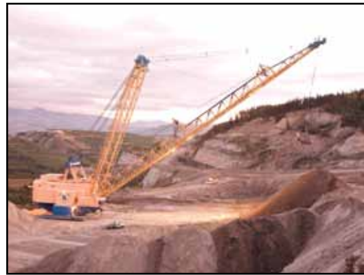
Photo of the “drag line” in action at the Usibelli mine. The massive machine removes overburden with a capacity rate of 30 to 40 cubic yards. For scale, a pickup truck is visible at the base of the drag line that was named by local students as “Ace in The Hole.” Photo by Chris Arend.
