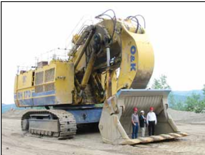
The shovel capacity of a loader is demonstrated by the people for scale. Photo by Chris Arend.
