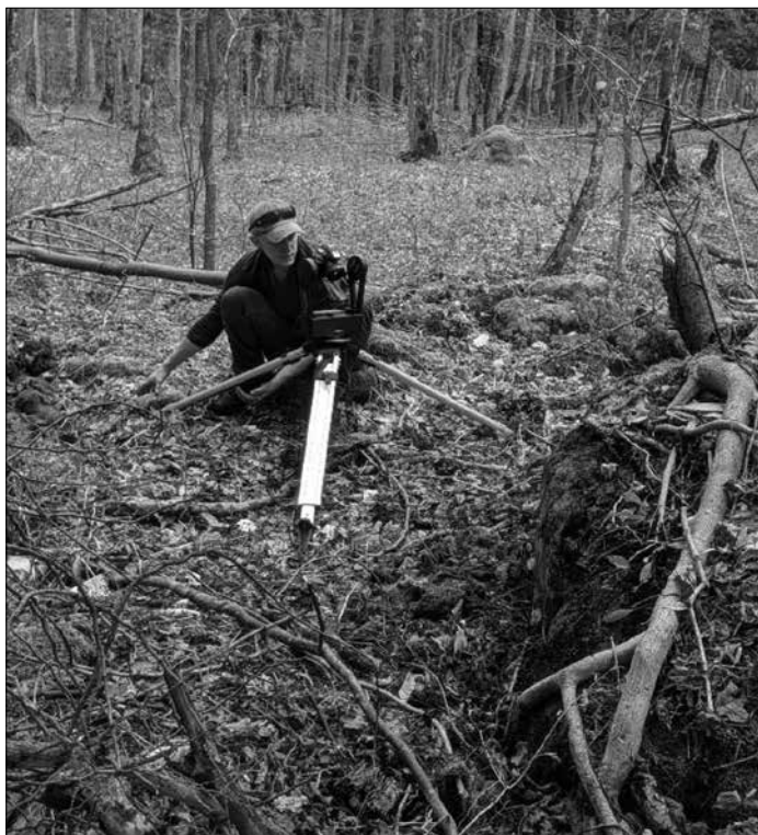
Figure 1. The robotic camera system setup with the system mounted on a tripod. Note that tripod mounting of the system does not allow for overhead imaging.
