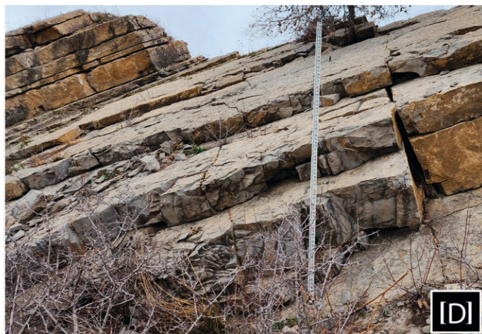
Figure C. Outcrop location of Kaibab Limestone in Holbrook, Arizona, showing heavy fracturing from weathering. Beds are near horizontal at the sample site (Davey, 2022).
