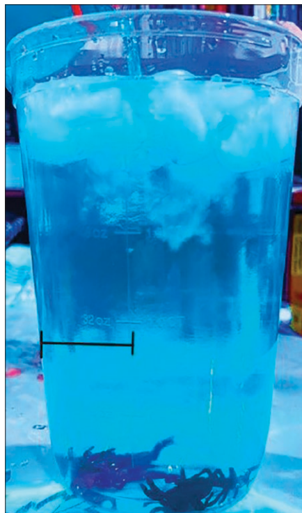
Figure 2. Brinicle Formation in the laboratory. As the dense brine water infiltrates downward, the brinicles begin to form and spread vertically to the bottom of the tank. Bar scale = 8cm.
