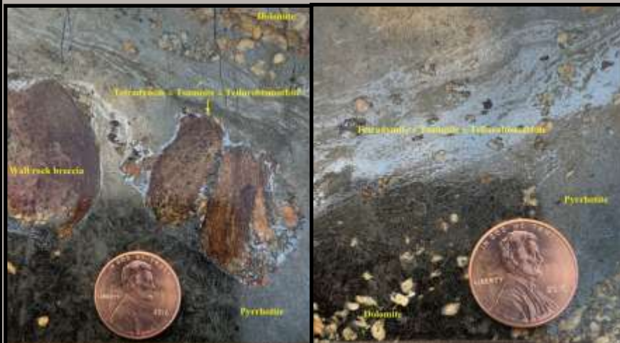
Figures 2 & 3—Lead grey-silvery colored tetradymite ± tsumoite ( \text{BiTe} ) ± tellurobismuthite ( \text{Bi}_2\text{Te}_3 ) fine veinlets in massive pyrrhotite (dark colored) + dolomite (brownish white) + wall rock (dark brown) from the deposit (sample #: SD34, Ore body #I-1 in Drift 3) and sample #: SD40, Ore body #I-1 in Drift
