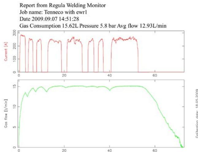
FIGURE 3. UNREGULATED GAS FLOW CONSUMPTION.
