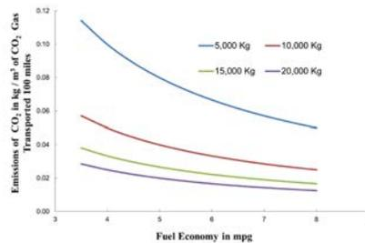
FIGURE 2. EMISSIONS FROM SHIELD GAS TRANSPORTATION IN CO<sub>2</sub> IN (KG/M<sup>3</sup>/100MILE).
