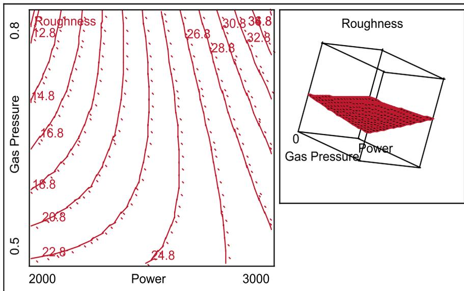
The contour plots indicated there were extensions of the desirable regions outside the range of factors settings selected for this study. In the *power \* feed rate* contour plot (*Figure 1*), a possible region was observed in the area below a *power* setting of 2000W.
