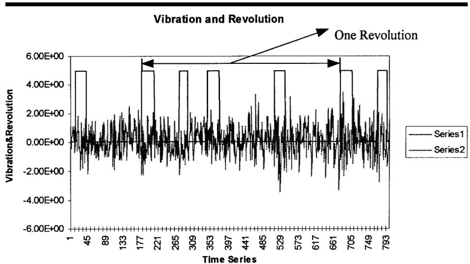
Figure 3. Original X Vibration under feed rate 2 ipm
