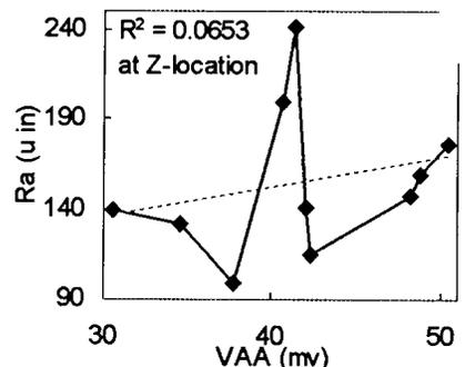
Figure 5. The relationship between the surface roughness (Ra) and the vibration amplitude average (VAA) at different locations.
