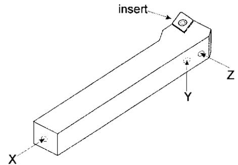
Figure 2. X, Y and Z Direction in Experiment
