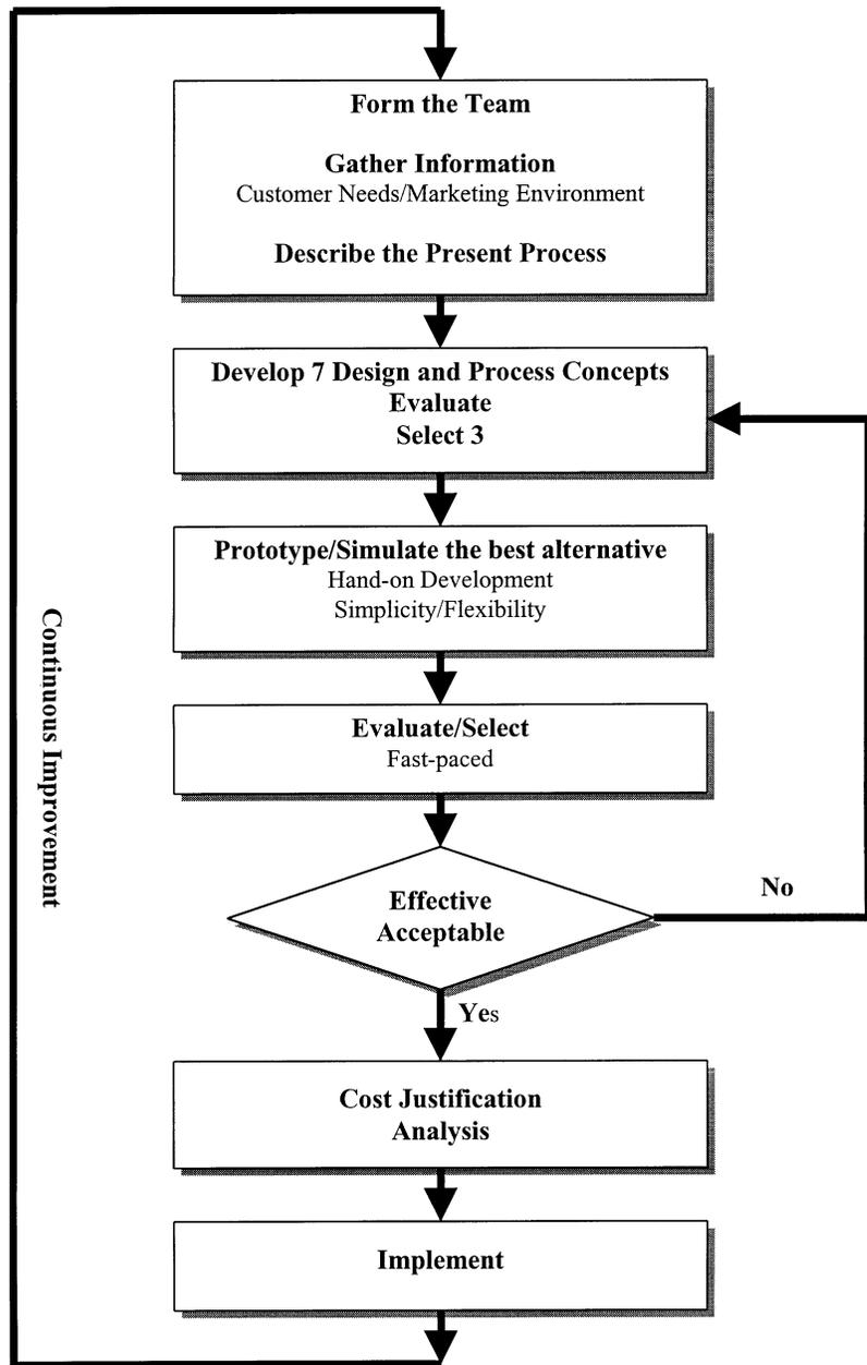
Figure 1. Flow chart of Kaizen procedure
