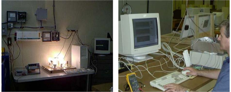
Figure 4. AC voltage divider and true RMS current transducer.
