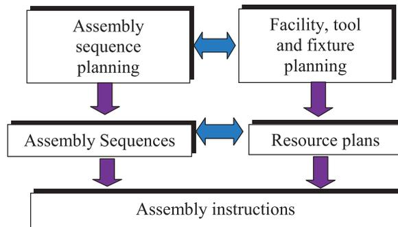
Figure 2. The architecture for assembly production optimization
