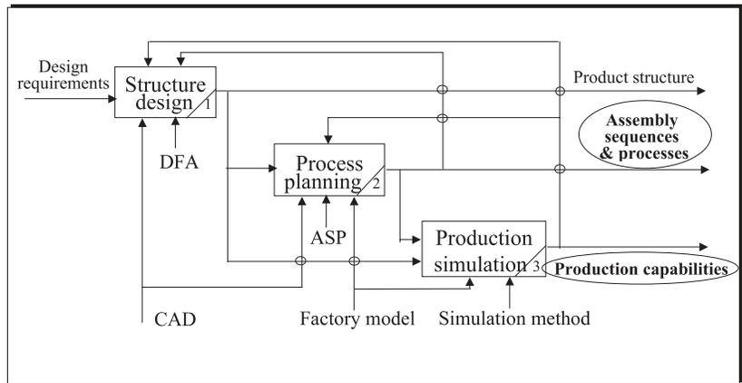
Figure 7. Structure design (IDEF0\_A11)
