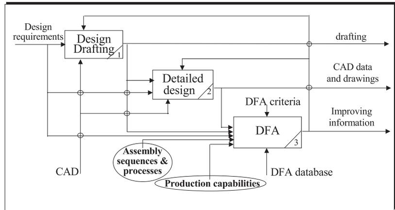
Figure 8. Assembly process planning (IDEF0\_A12)
