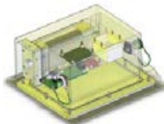
Asset monitoring unit
