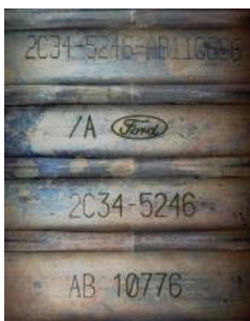
Figure A8. Converter dot peen (top) and laser etch (bottom) after thermal cycle
