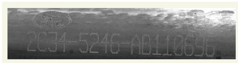
Figure 3. Example of a part with mechanical dot peen marking
