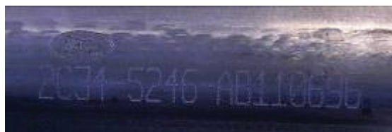
Figure A4. Close-up view of dot peen marking
