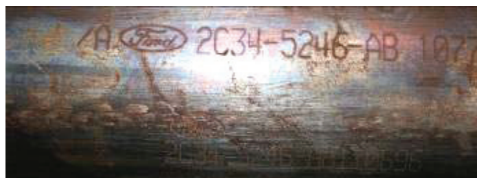
Figure A9. Pipe laser etch (top) and dot peen (bottom) after salt fog exposure
