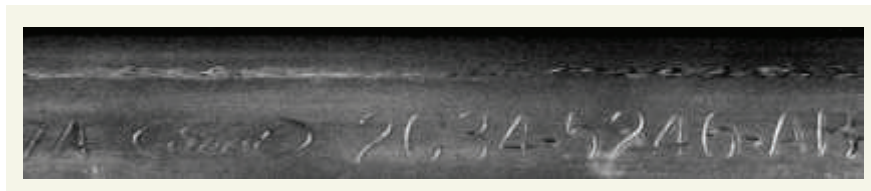
Figure 2. Example of a roll stamped part
