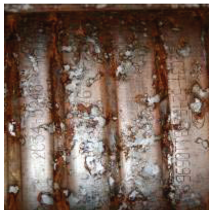
Figure A7. Converter laser etch (left) and dot peen (right) after salt fog exposure
