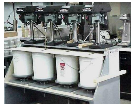
Figure 2 – Laboratory Set-up to Maintain Agitated Recycled Water Slurry
