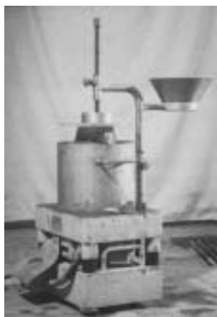
Figure 9.4 The Vebe test
