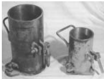
Figure 9.7 Restrained rubber capping system
