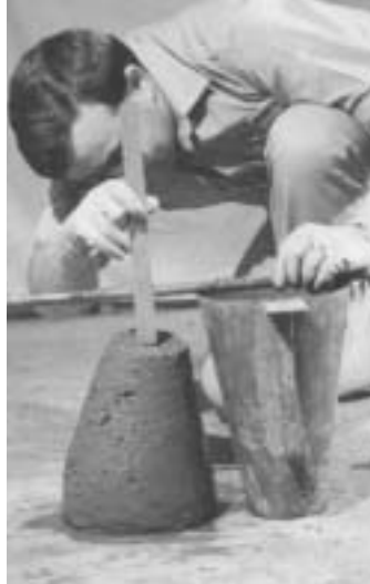
Figure 9.1 The slump test
