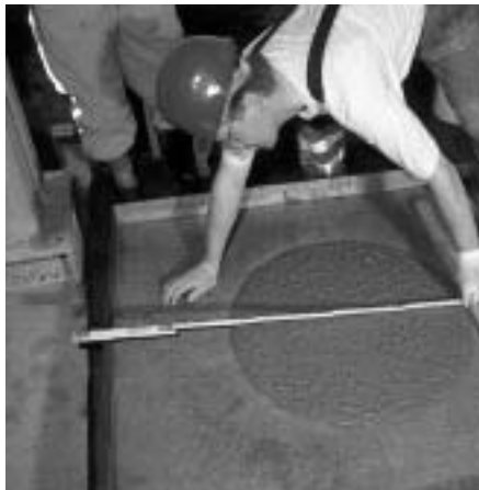
Figure 9.3 The spread test
