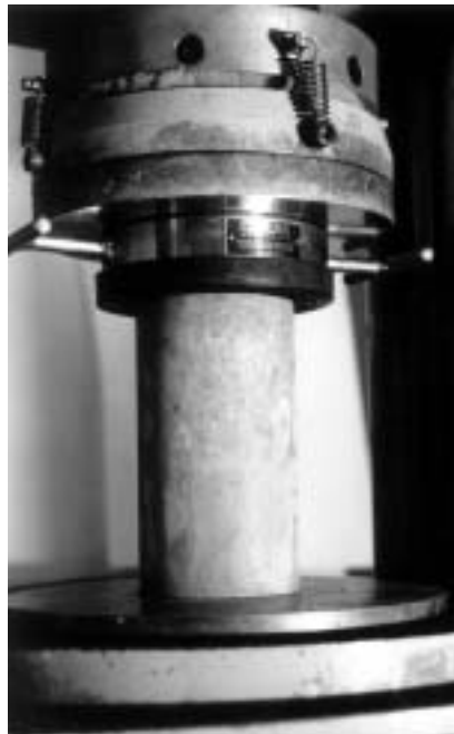
Figure 9.7 Restrained rubber capping system
