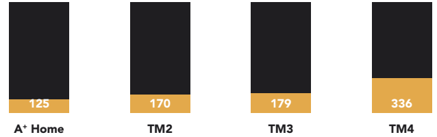
Overheating in hours pa (hours exceeding 26°C, living room shaded by sliding sun shutters)
