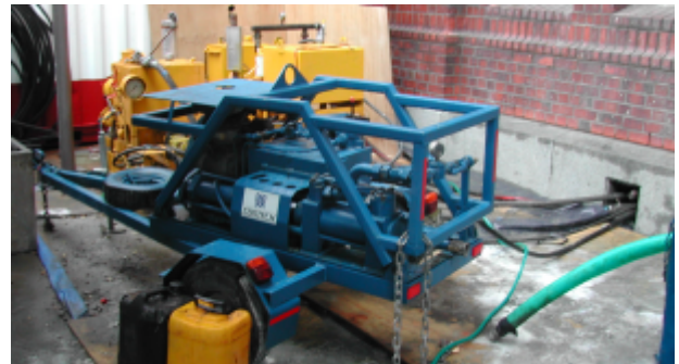
Figure 11: High pressure grout pump
