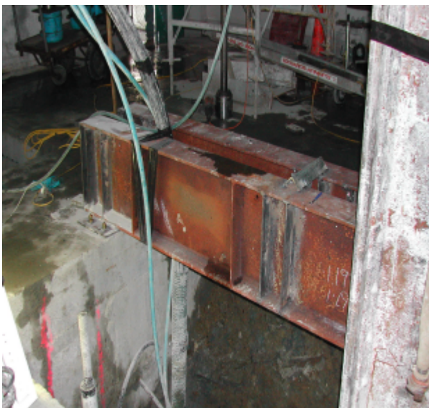
Figure 3: Reaction frame for 1700kN proof test
