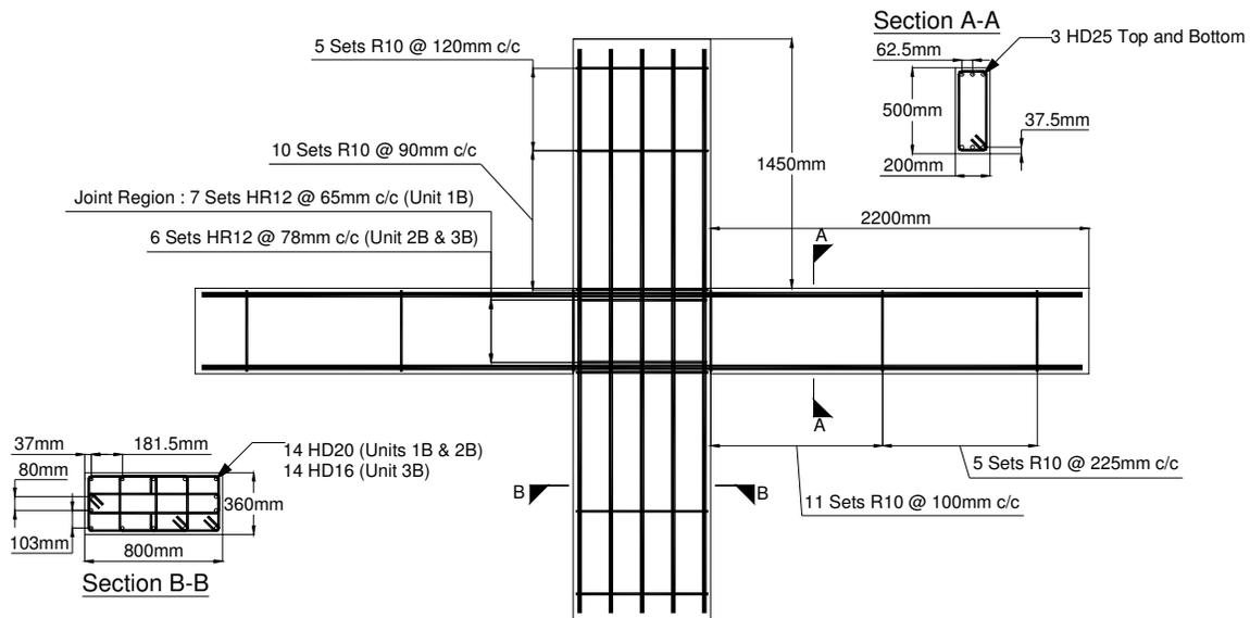
**Figure 4 Principal dimensions and reinforcement plan of unit 1B (Brooke)**
