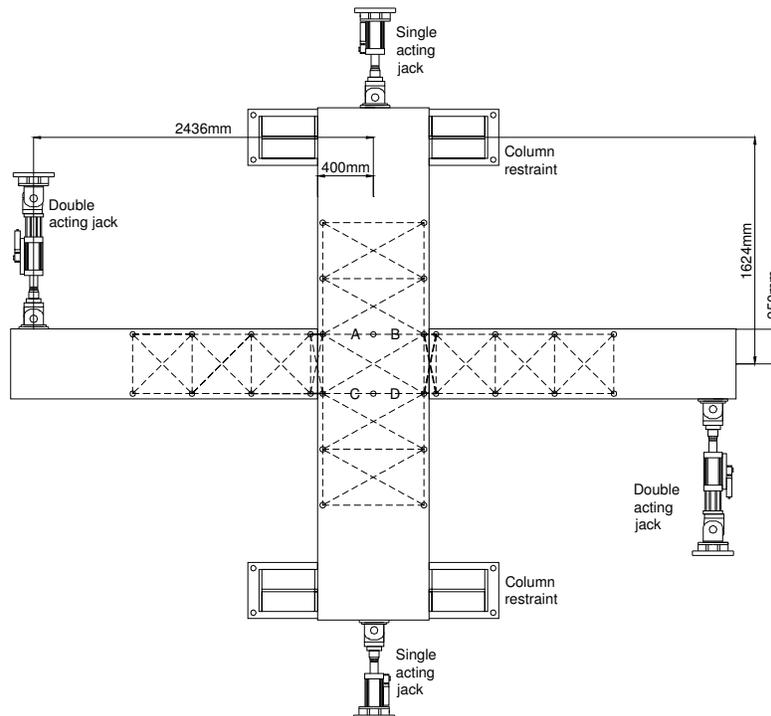
Figure 5 Portal gauge layout and loading arrangement for unit 1-3B.
