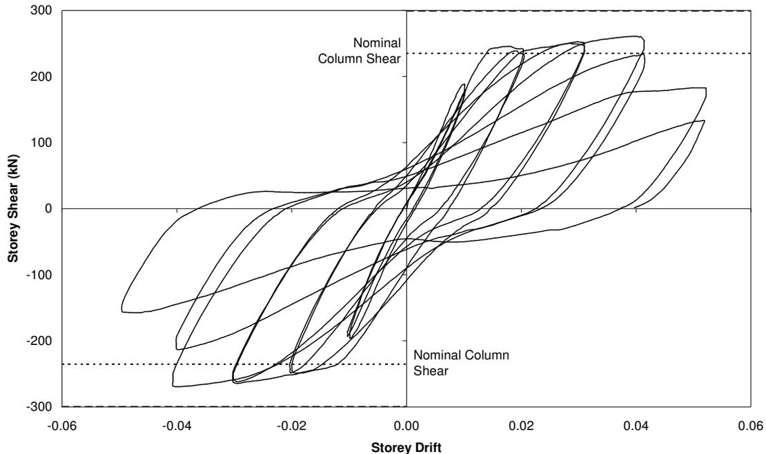
**Figure 9 Unit 3B storey column shear versus storey lateral drift.**
