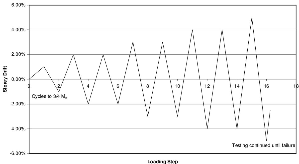
**Figure 6 Planned loading cycle for units 1-3B**
