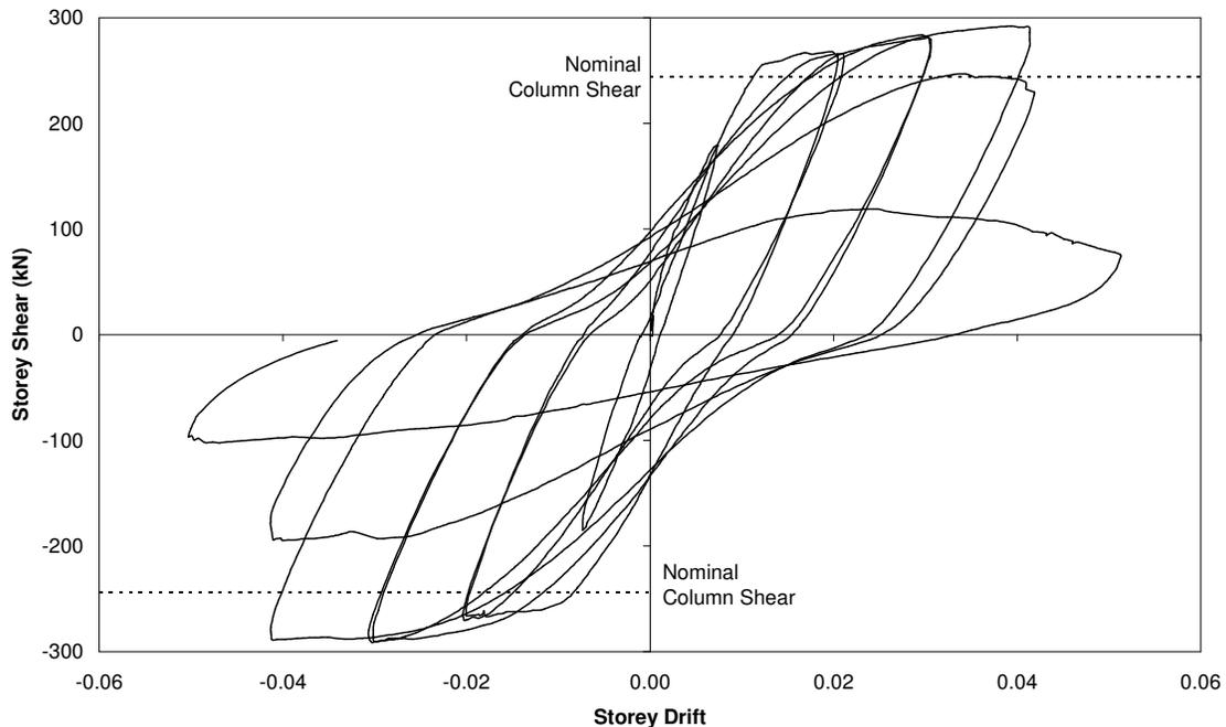
**Figure 8 Unit 2B storey column shear versus storey lateral drift.**
