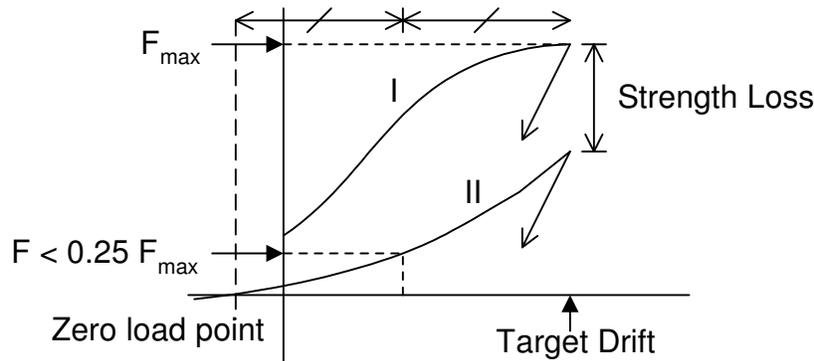
**Figure 1 Criteria used to determine occurrence of bond failure.**
