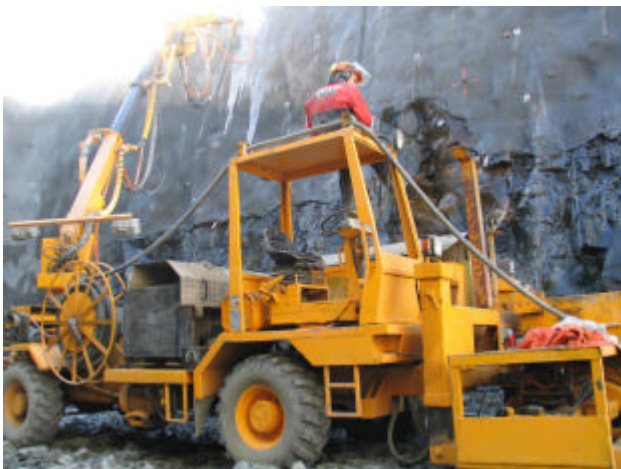
Figure 4: Conventional shotcrete rig for rock consolidation and tunnelling support
