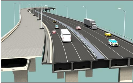
Stage 1 – Construct new southbound viaduct
