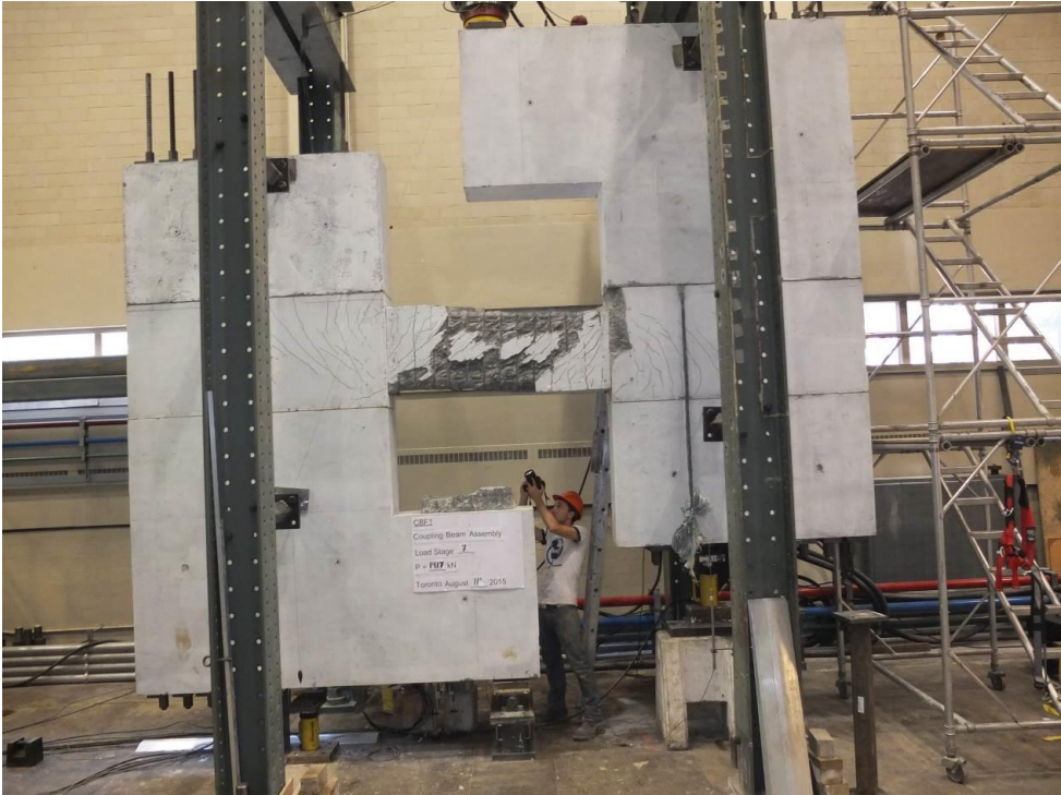
Figure 13. Specimen CBF1 after failure, V_{max} = 1918 kN, right wall pushed down 70 mm.
