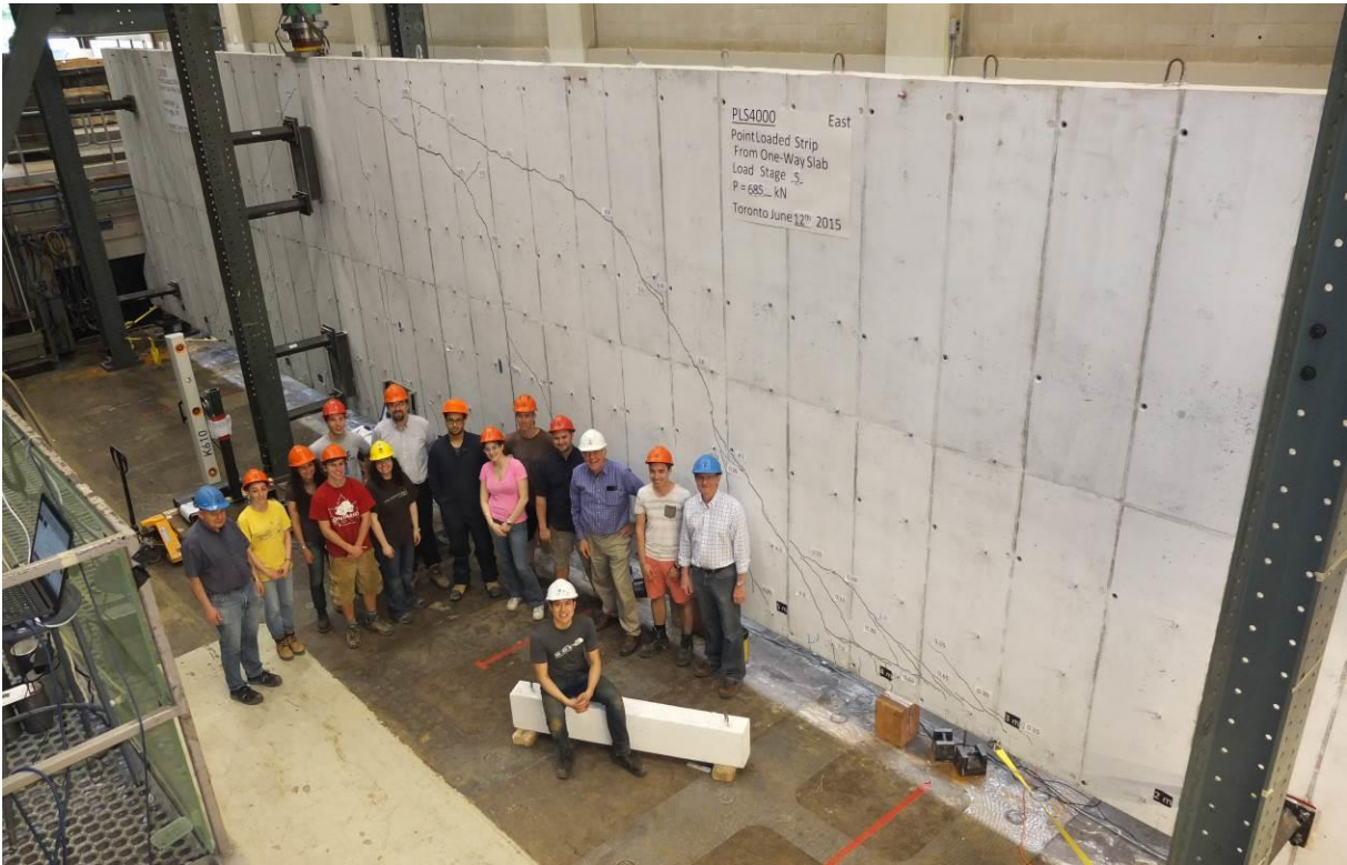
Figure 2. Strip from four metre thick slab and 300 mm deep traditional size shear specimen
