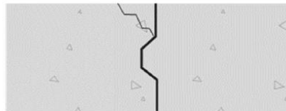
Figure 10. Keyjoint – risk of cracking under heavy loads
