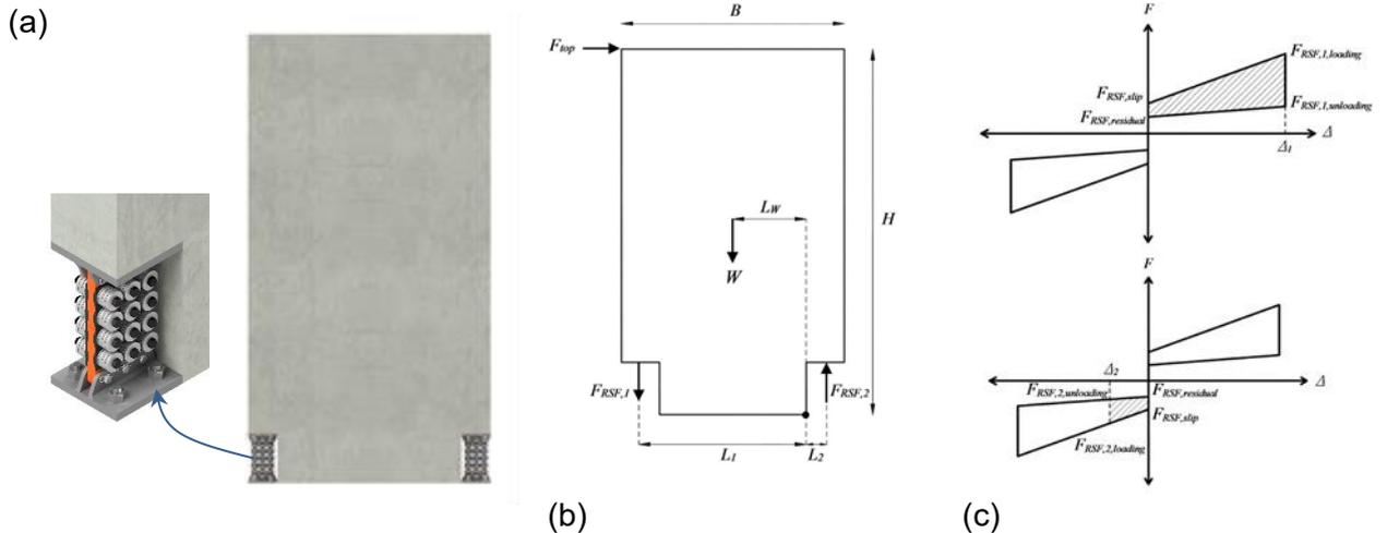
Figure 5: Proposed rocking shear wall: a) RSFJs adopted as hold-downs, b) Free body diagram of the wall
