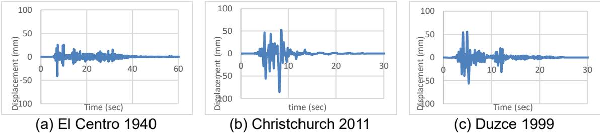
Figure 10: Roof displacement demand for selected ground motions
