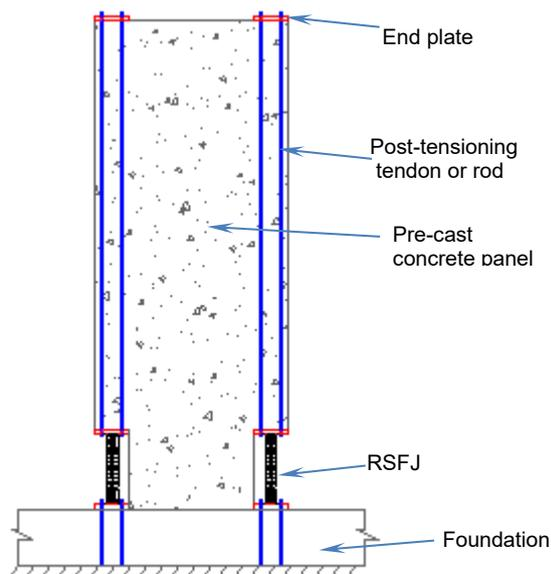
Figure 7: different components of the proposed rocking pre-cast concrete wall system
