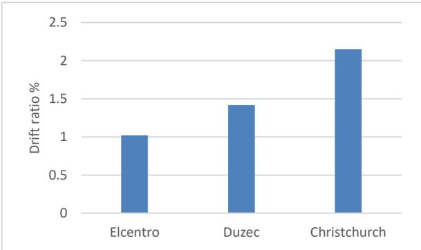
Figure 12: Maximum floor drift ratio for the selected earthquake events
