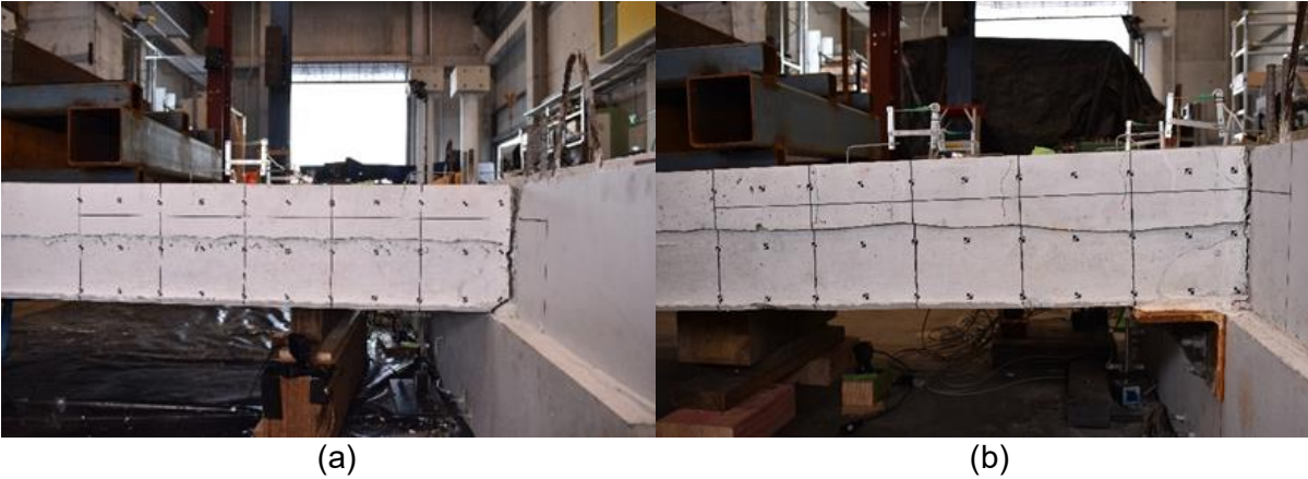
Figure 7: Specimen 1 Residual Crack After ±4.5% Drift (a), Specimen 2 at -2.75% Drift (b)...
