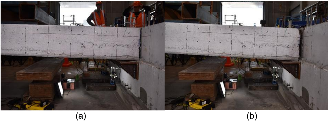
Figure 12: Specimen 6 at +3.0% Drift (25 mm Pull-Off) (a) and at +4.5% Drift (b)
