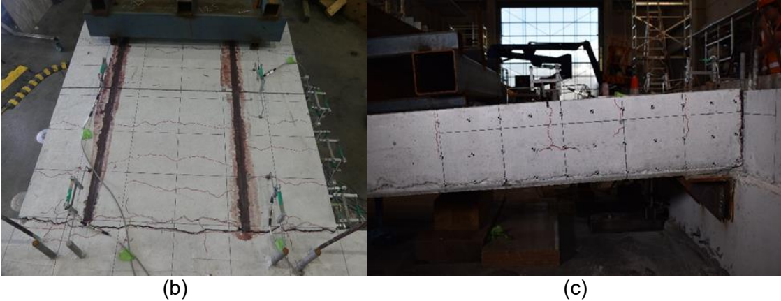
Figure 10: Test 5 Load-Drift Plot (a), Topping at -4.5% Drift (b) and at -6.0% Drift (c)
