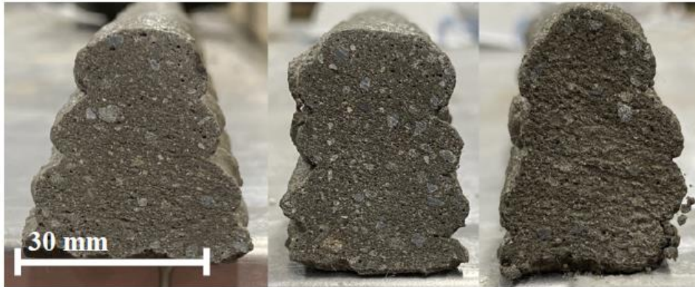
Figure 7 Visual inspection of the filament cross-section (Mix 1 on the left, Mix 2 on the centre and Mix 3 on the right image)
