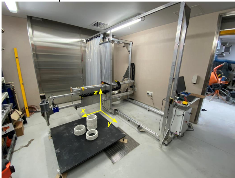
Figure 2 The UC custom-built 3D concrete printing machine.
