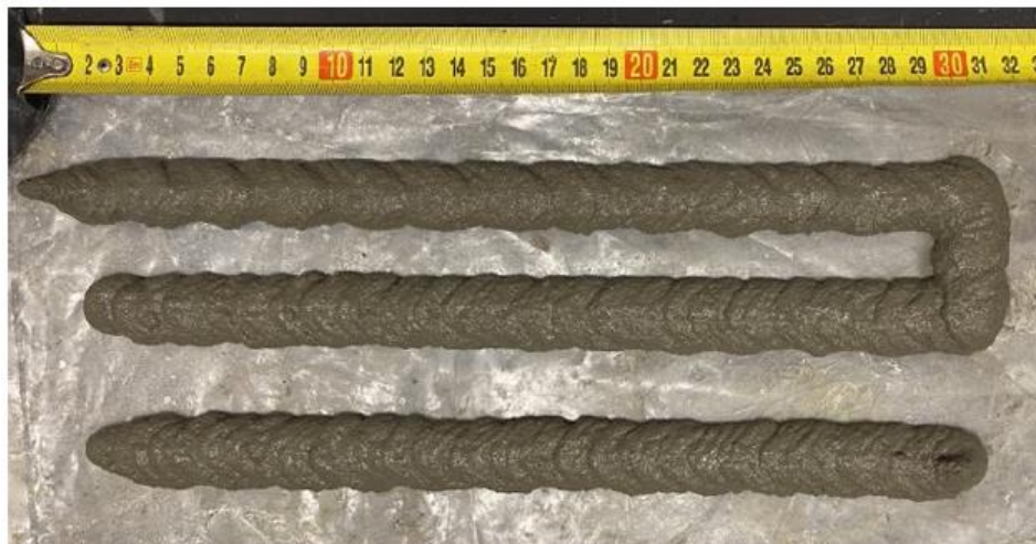
Figure 5 Mix 2 with PVA extrudability test trial one.
