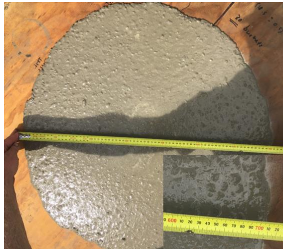
Figure 3. On-Site Flow Test of Trial Self-Compacting Concrete Mix
