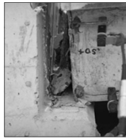
Figure C18.8 - Precast rib not restrained by support member
