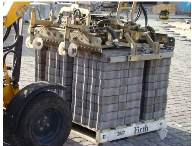
Figure 29: Paver Laying Machine
