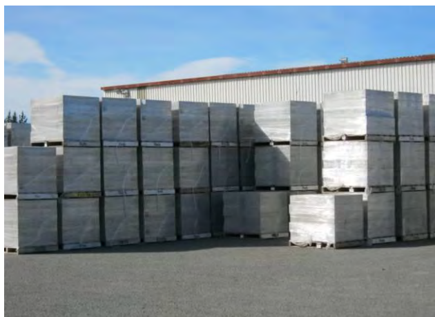
Figure 35: Cubed Pallets of Concrete Blocks
