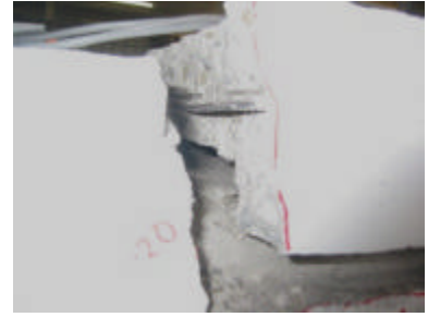
(c) Close up showing the topping separation
