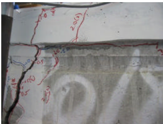
Figure 5-5. Cracks in the topping at -3.0% (-2.89%) drift
