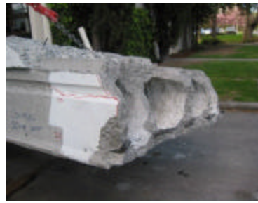
(f) The end of the hollowcore unit after removal. Note the kinked prestressing strands.
