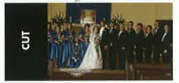
16x9 Content (right screen pan & scan) as displayed on a 4x3 monitor (cuts out 3.5 bridesmaids)
