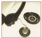
headphone to the middle left and the loudspeaker in the middle (with the two wires connected to it). The connecting Terminals are easy to spot and are connected to the Voice Coil inside the Dome cover.
