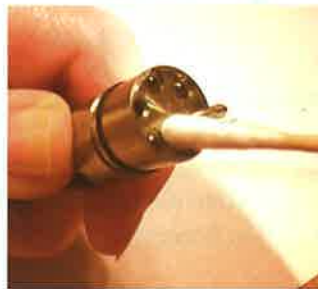
Figure 6: Expanded Beam (EB) connector lenses can be cleaned with a lint-free swab (left photo) and inspected with a 10x eye loupe (right photo).
