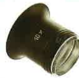
Figure 6: Expanded Beam (EB) connector lenses can be cleaned with a lint-free swab (left photo) and inspected with a 10x eye loupe (right photo).
