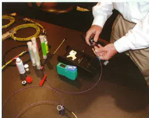
Figure 8: Field test tools can include a camera probe and video display (black test unit) that provides the ability to clip onto a PC terminus while still in the connector (right photo). The blue box in the middle of the left photo is a box of lint-free cleaning wipes, and the white and blue unit in the right photo is a calibrated light source. These tools are supplied by Noyce as well as others.
