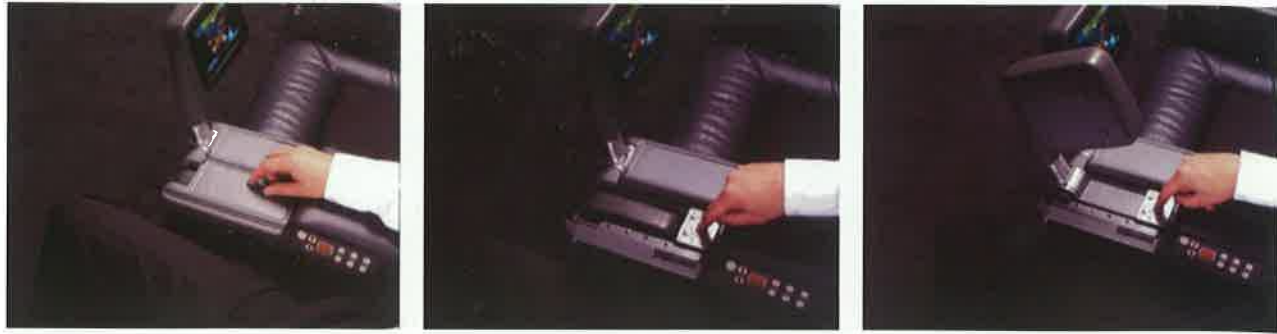
Functional prototype for the United Airlines/GEC Marconi LCD video monitor console and handset stowage
