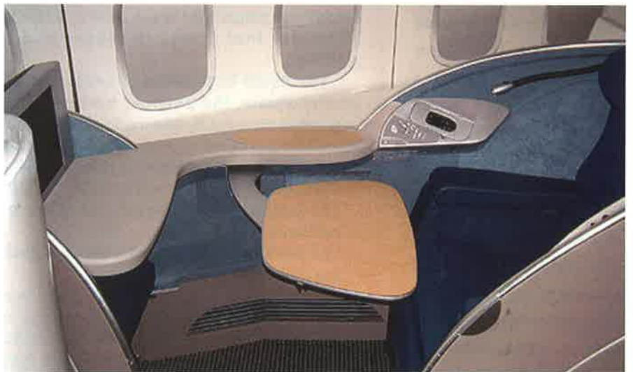
Dining table stows under the video counter and effortlessly articulates aft to the precise dining height. It can be simply be pushed forward for entry and exit from seat.
