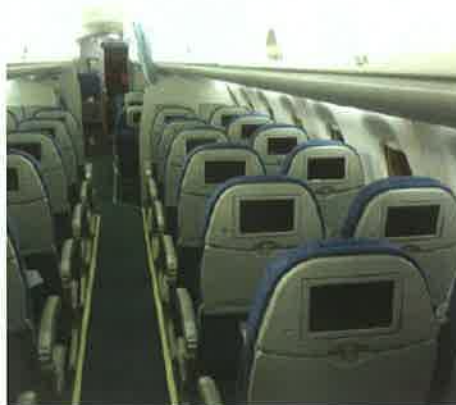
Inseat Interactive/Video-on-Demand IFE system on an Embraer EMB 175 Aircraft
