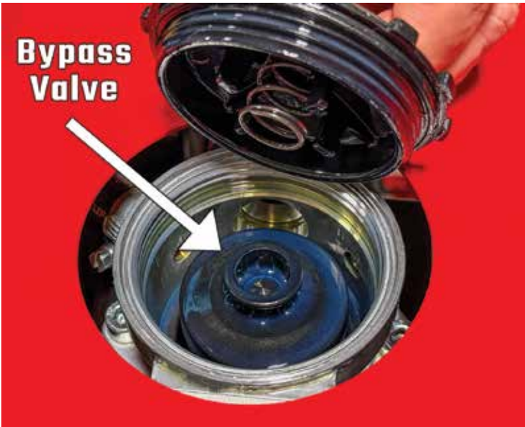
Many of the return line filters have a bypass valve to keep the system operating and minimize the back pressure.
