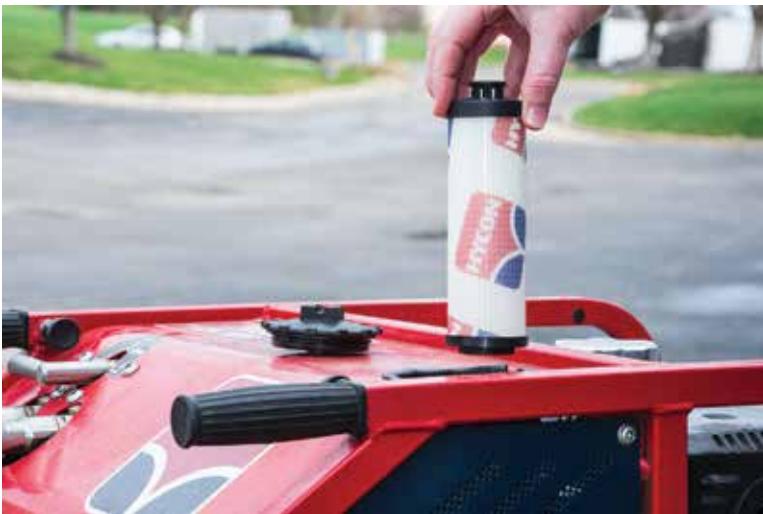
It is important to perform regular maintenance on the power pack to include changing the filter.
