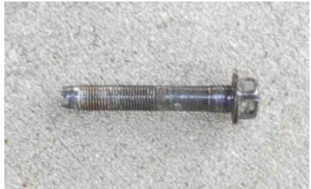
**Figure 1 – A Typical Blade Shaft Thread (Bolt)**
