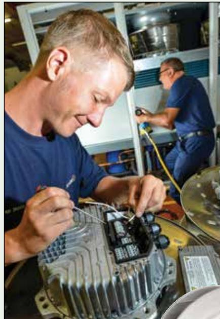
*Above: Controls logic being integrated into an EC fan*
