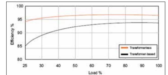
Fig 1: Transformerless and transformer-based UPS efficiency/load curves
