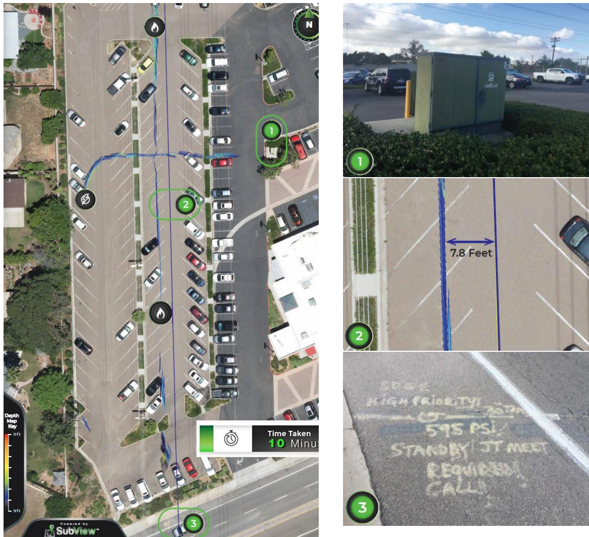
Figure 5—The map in SubView reveals a shallow electrical line that crosses over the pipeline (1). The transmission pipeline lies approximately 7.8 ft to the west of the position in the SDG&E map (2). The pipeline's location lines up with paint markings in the street from a recent locate (3).
