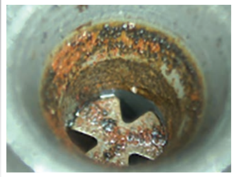
Excessive amounts of water was found in the fuel tank.
