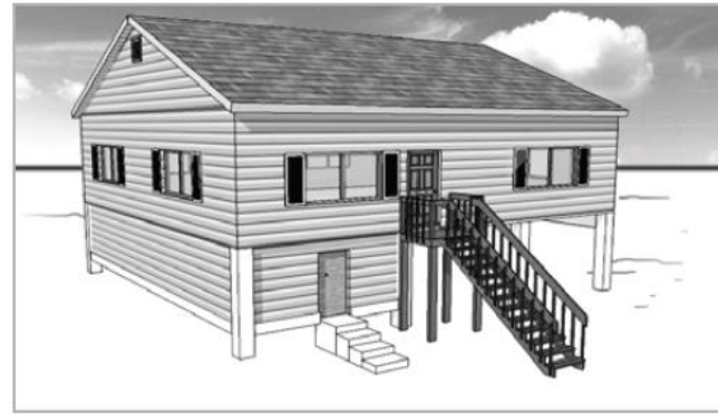
Elevated hanging floor
