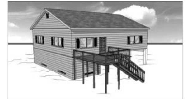
Elevated on posts, piles, or piers with a properly vented partial enclosure
