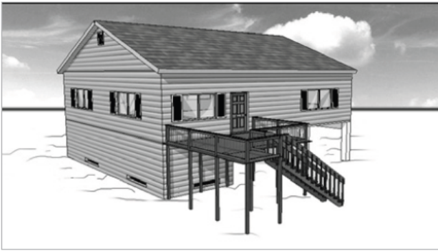
Elevated on posts, piles, or piers with a properly vented partial enclosure
