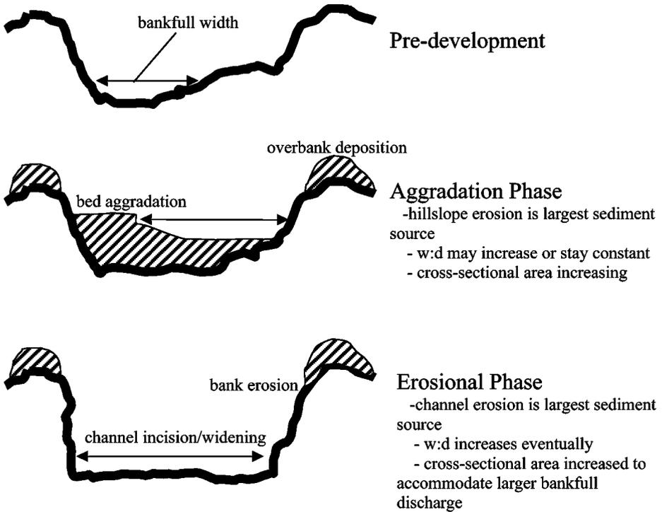
**Figure 2** Channel changes associated with urbanization. During the construction phase of urbanization, hillslope erosion increases sediment supply leading to bed aggradation and overbank deposition. After construction ceases hillslope sediment supply is reduced, but bankfull flows are increased owing to increases in imperviousness. This leads to increased channel erosion as channel incision and widening occur to accommodate increased bankfull discharge.
