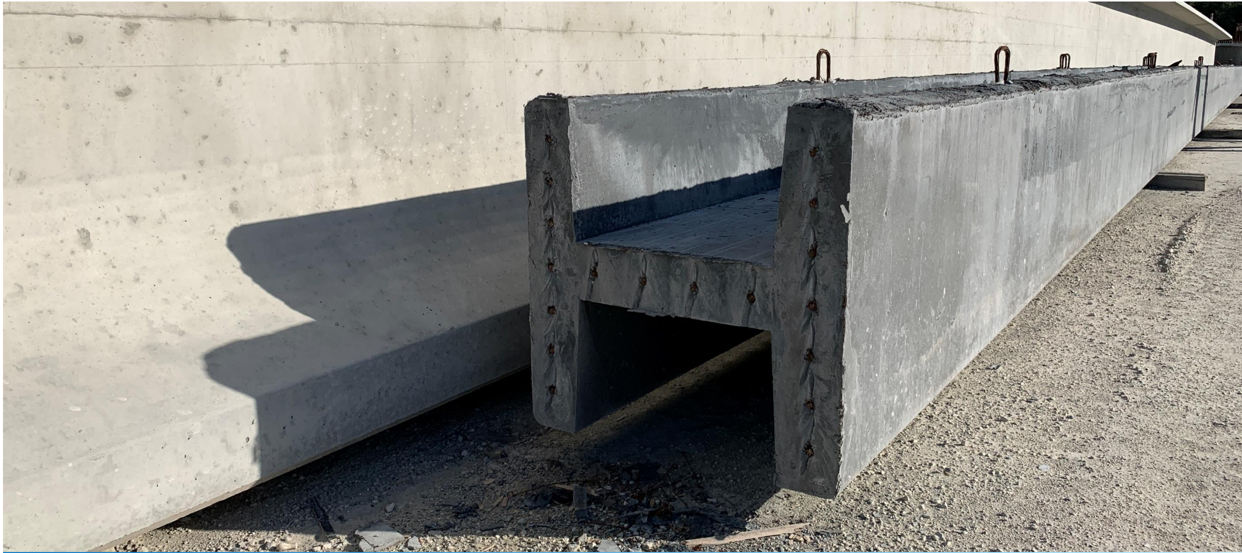
Pre-tensioned H-piling after casting at Dura Stress Inc.
