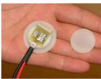
Wireless band-aid: peel-and-stick disposable detector that monitors vital signs
