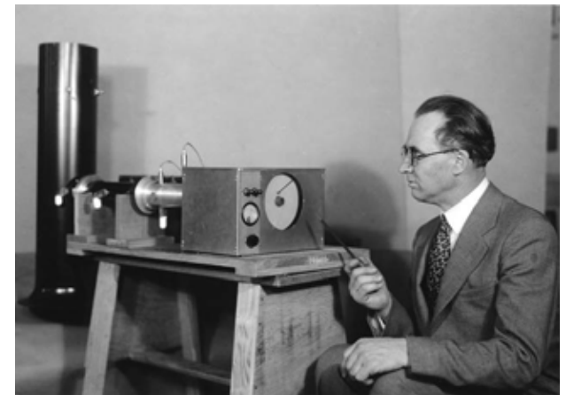
Oliver H. Gish with his electrical conductivity apparatus for the Explorer II manned balloon flight into the stratosphere in 1935. Image is courtesy of the Carnegie Institution for Science, Department of Terrestrial Magnetism.
