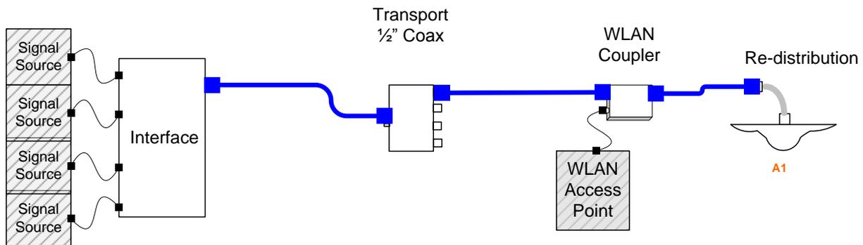
Passive systems are the least expensive type of system in smaller facilities. However, they require professional engineering design, due to installation complexities. Additionally, the power of the signal source needs to be stronger than in an active or hybrid coverage solution and this generally increases the cost of the signal source the MNO has to provide.
