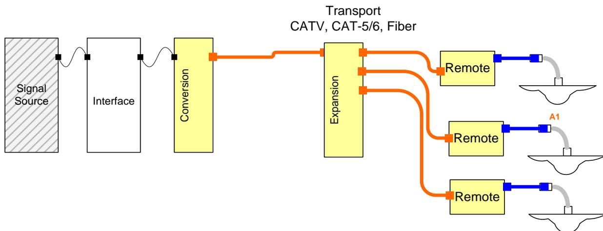
Active systems are best at providing coverage for a single MNO, grouping of MNOs, or grouping of services, such as cellular/PCS, and can be very cost effective. However, when a large number of MNOs or numerous services on a single MNO, such as cellular/PCS/LTE, then multiple “parallel” networks may be required. For a building, the actual design will be typically based on size, cost, output power, and antenna configuration option considerations.
