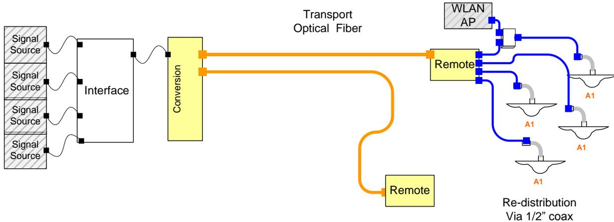
Like the active system, the hybrid system utilizes low-loss, fiber-optic transport and supports low-input power from the MNOs. This is a highly desirable feature, since it lowers the financial barrier for the MNOs. The passive part of the system supports the combining of various services at the remote hub location so that multiple services can be provided over a shared antenna.
