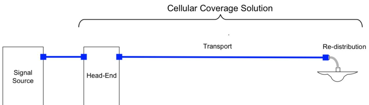
While simple in concept, cellular coverage solutions can differ in many ways and the industry has categorized them in the terms active, passive, and hybrid. These terms refer to the electronics or lack of electronics in the head-end and transport. Before covering the differences in these areas, it is useful to discuss some common elements – the transport cabling and re-distribution elements.
